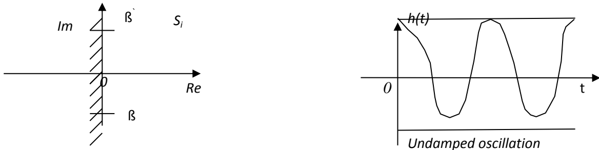
Fig.6.17a. Location of imaginary roots and the corresponding transient process
